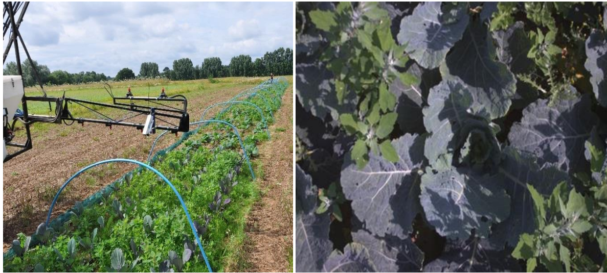
Figure 1. EyeWeed camera system mounted on the boom of a sprayer, capturing images of weeds and red cabbage crop (left). Image of a weedy plot with red cabbages as it was captured using EyeWeed (right). The hoops were to support fleece.
